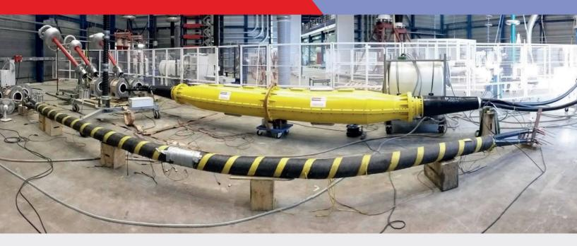
For the offshore repair of high voltage OWF subsea export cables damaged during installation or operation Power CSL offers its robust and reliable repair joint product.
