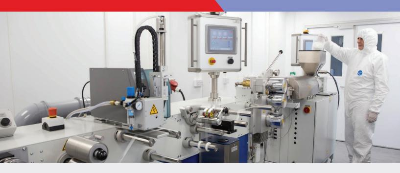
Power CSL operates modern tape extrusion facilities housed in an ISO Class 6 clean room for the production of materials for its factory jointing service.
